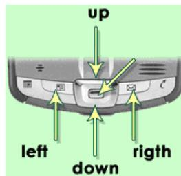
Fig. 2. The hardware buttons used to control the device
